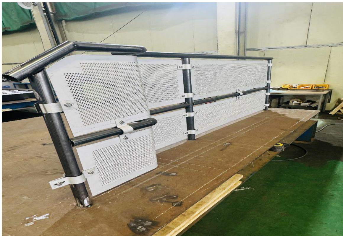
**MTE Handrail Infill Panels, Wind - Radiated Heat and Dropped Object Protection.**
